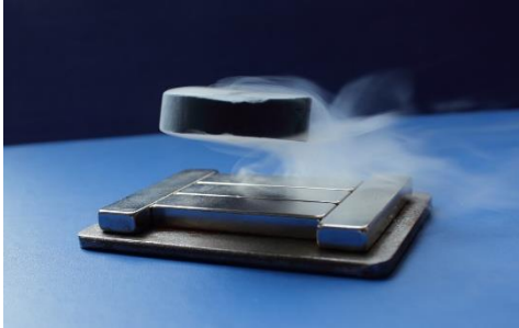
Levitation of a magnet above a superconductor (Stephen Blundell and Andrew Boothroyd)
