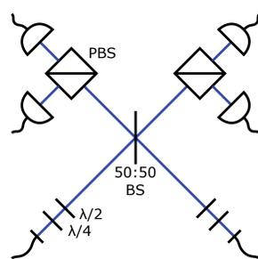
To create ion-ion entanglement, we interfere the photons emitted simultaneously from each ion on a 50:50 beamsplitter. The two-photon state is measured using a four detector scheme, probabilistically heralding the projection of the ion-ion state into a  $\Psi^+$  or  $\Psi^-$  Bell state, dependent on the detector click pattern.
