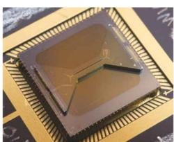
We have constructed two identical vacuum systems, each containing a HOA2 linear multi-zone surface trap (courtesy of Sandia National Labs), designed to operate with both  $^{43}\text{Ca}^+$  and  $^{88}\text{Sr}^+$  and allow high-fidelity mixed species gates.
