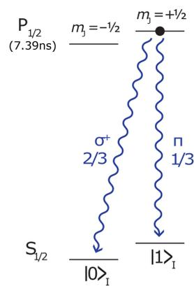
We need to generate photons entangled with our ion qubits in order to implement our ion-photon network. We do this by exciting a  $^{88}\text{Sr}^+$  ion to one of its short-lived  $P_{1/2}$ -states using a picosecond laser. The emitted 422 nm photon is entangled in frequency and polarisation with the resulting Zeeman qubit.
