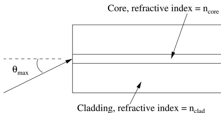
Light may only be transmitted along the fibre if the incident angle of the light is less than a maximum angle  $\theta_{\text{max}}$ . By using your equation from above and Snell's Law, or otherwise, derive an expression for  $\theta_{\text{max}}$  in terms of the core and cladding refractive indices only.
