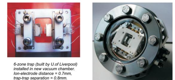
6-zone trap (built by U. of Liverpool) installed in new vacuum chamber. Ion-electrode distance = 0.7mm, trap-trap separation = 0.8mm.
