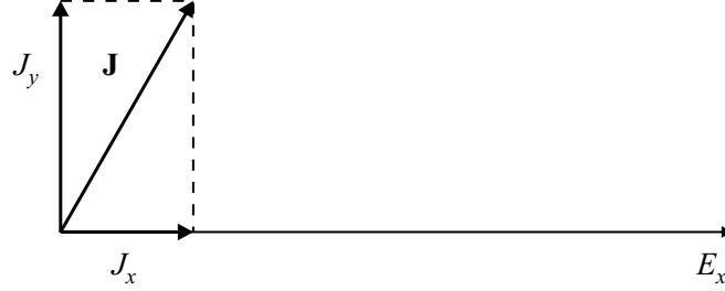
Figure 11.2: Geometrical interpretation of the components of current density J_x , J_y and caused by electric field component E_x and magnetic field (0, 0, B) ; \mathbf{J} is the total current density.
