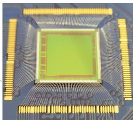
The collaboration has recently produced a prototype device which uses an array of 72x72 intelligent pixels, inspired by technology originally developed for use in detectors for
