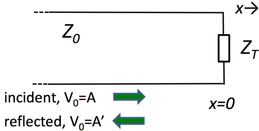
Figure 5.4: A transmission line that is terminated at x = 0 by an impedance Z_T .
