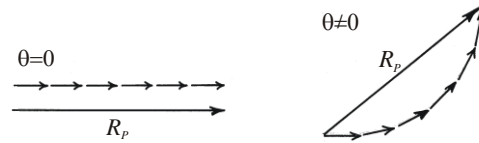
Figure 1.8 (a) Phasor diagram for finite slit showing resultant R_p for \theta=0 and \theta \neq 0
