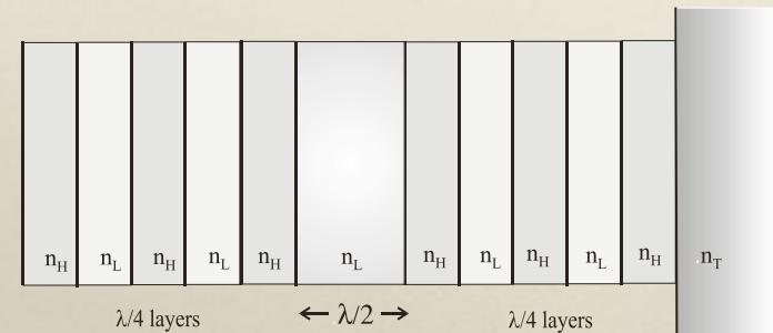
Interference filter; composed of multi-layer stacks
